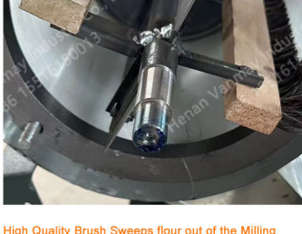
High Quality Brush Sweeps flour out of the Milling Room, Which Increases the Milling Efficiency.
